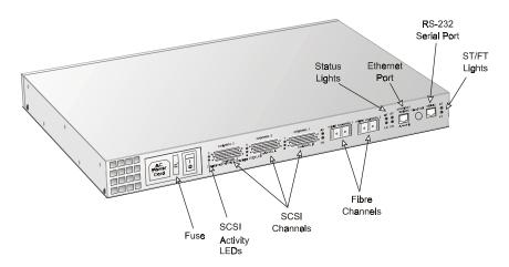
Figure 2-3. Rear panel components
